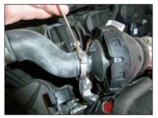
5. Release the one-time use clamp that secures the sound tube to the drum and then disconnect and remove the sound tube from the vehicle.
