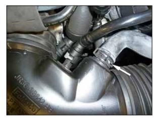
4. Release the spring clamp that secures the sound tube to the intake tube fitting and then disconnect the sound tube from the intake tube.
