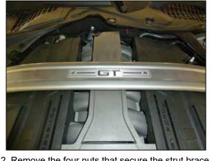
2. Remove the four nuts that secure the strut brace and then remove the strut brace from the vehicle.
