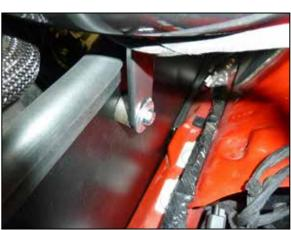
15. Install the AEM® intake tube into the coupler at the throttle body and onto the rubber mounted stud in the heat shield. Adjust the tube for best fit and then secure with the provided hardware and hose clamp. Connect the crankcase vent and EVAP vent lines.
