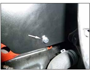
12. Install the heat shield assembly into the vehicle and secure to the factory air filter housing mounting location and to the frame rail using the provided hardware.
