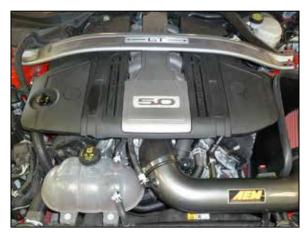
18. Reinstall the decorative engine cover and strut bar, secure with the factory hardware.
