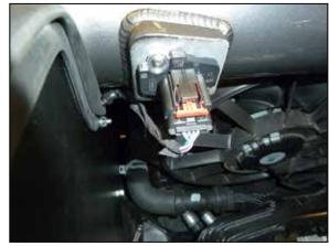
16. Connect the mass air sensor electrical connection.
