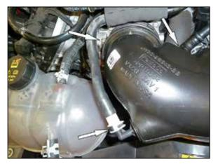
6. Disconnect the vent lines attached to the intake tube. Loosen the hose clamps that secure the intake tube to the air filter housing and throttle body and then remove the intake tube from the vehicle.
